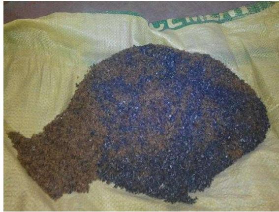
Fig .2 Lathe scrap powder partial replacement with sand
