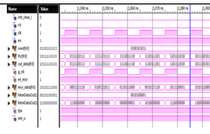
Figure 12: Top module output of Existing method which shows circuit is faulty.
