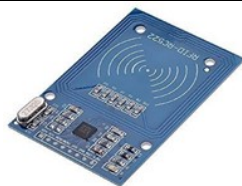
Fig- 3: RFID reader.
